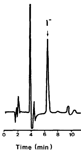
Fig. 5. Ion chromatographic determination of iodide in a whole milk extract. Conditions: Vydac 302 IC column, 6.5 \text{ mM} \text{KH}_2\text{PO}_4 (pH 6.3) at 2 \text{ ml/min} ; amperometric detection (Ag, +0.155 \text{ V} ). From ref. 68.
